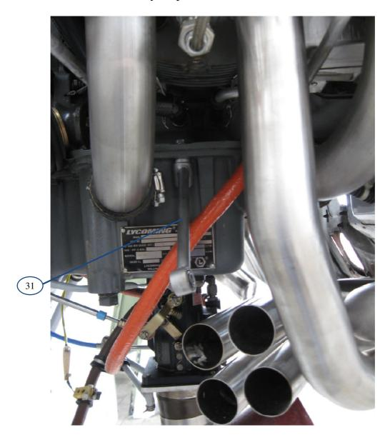
7 - Apply high temperature grease to the inside of 4 in 1 tube.
