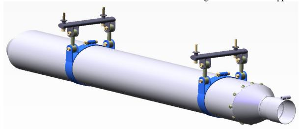
18 - Position the double swivel-joint tube on the 4 in 1 tube, Position the muffler and make sure that the swivel-joints are lined.
