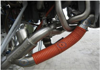
Orient the cabin-heat box to ensure that the flexible ducting are correctly positioned and do not in contact with any of the primary tubes.
