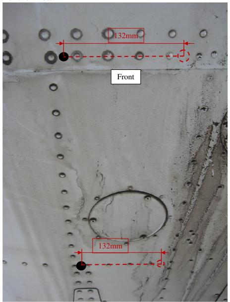
13 - Remove the trapdoor under the cockpit.
