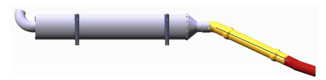
19 - Position the lower cowling and make a cut to ensure that the exhaust isn't in contact with the cowling.
